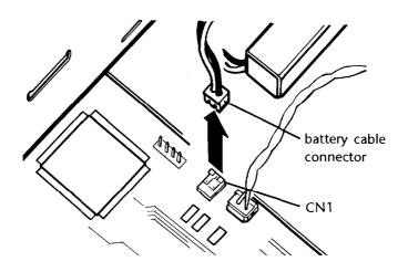
2. The battery is attached to the computer with Velcro? Remove the battery by pulling it up from the bottom of the computer case, as shown below. Then set it aside.
